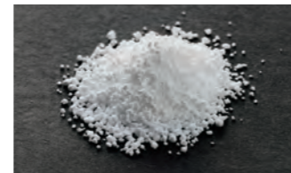
Polyphenylene sulfide (PPS) Kureha's PPS has excellent mechanical strength, heat resistance, chemical resistance and flame resistance, and is highly regarded worldwide as a super engineering plastic.
